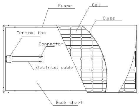
Figure 1 the components of a module
