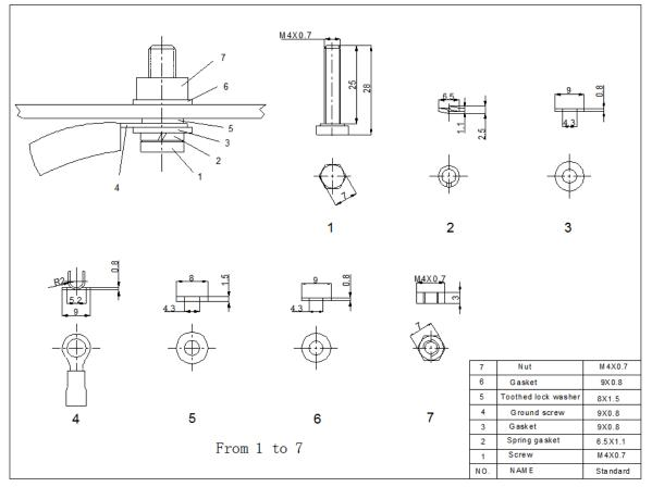
Figure 4.Example of acceptable ground connection
